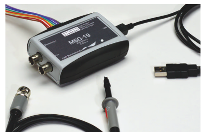
The MSO-19 lets you view one analog and eight digital signals.
