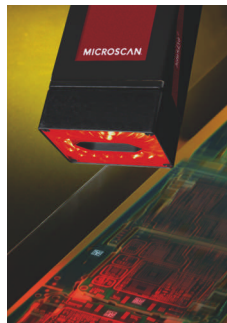
A HawkEye smart camera reads 2-D symbols on PCBs.
