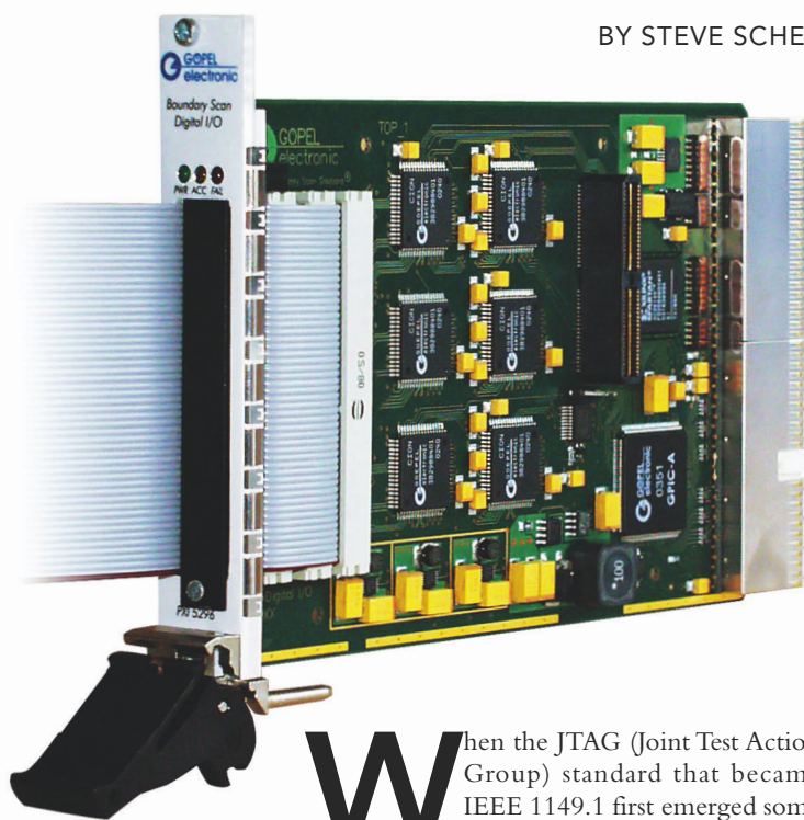
FIGURE 1. Boards like this Mixed Signal I/O Module PXI 5296 that plugs into the PXI bus can turn a conventional PC into a multipurpose test instrument.
